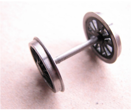
Tender wheels assembled with no spacing washers.
